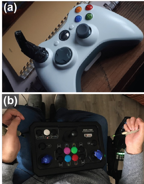
Figure 3.5: (a) The controller P12 modified to make its joystick easier to use. (b) The custom controller created for P10 as an accessible substitute for other game controllers.
